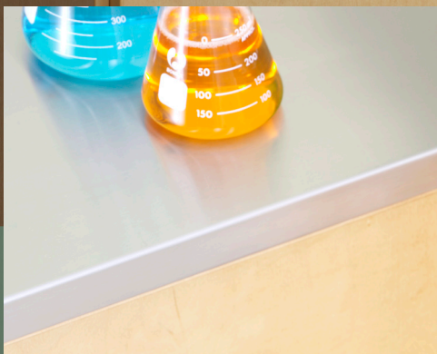
Square edge: All table and countertops are constructed of 16 gauge stainless steel and polished to a #4 finish.
